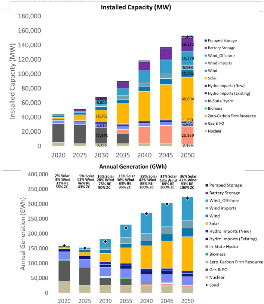
By 2050, across all modeled pathways, New York installs over 60 GW of solar capacity (both utility-scale and distributed resources), between 16-17 GW of new land-based wind capacity (including imported wind from neighboring ISOs), and between 16-19 GW of offshore wind resources, illustrated in Figure 30.
